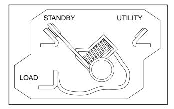
Figure 3. Load Connected to Standby Power Source
